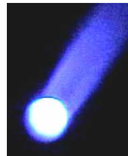
0.3 mm platinum ball being bombarded with laser energy to form up on the end of 30 gage wire under magnification.
