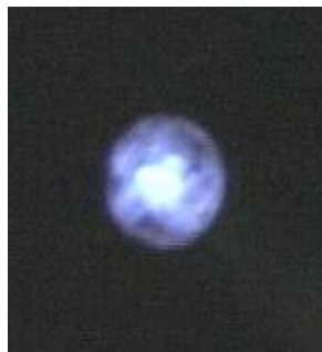
0.3 mm platinum ball being bombarded with laser energy to form up on the end of 30 gage wire under magnification.
