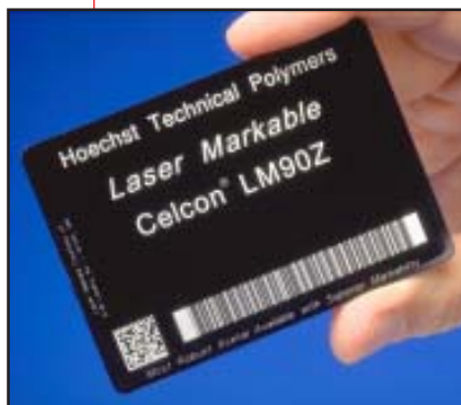
Figure 2. High-resolution, high-contrast markings can be etched by industrial lasers in parts molded in Celcon LM90 and LM90Z acetal copolymer.
