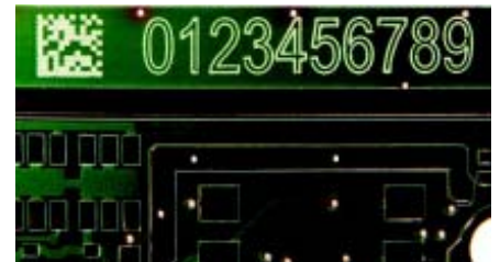
Fig. 1. DataMatrix marking with CO 2 lasers. The laser radiation is absorbed by the soldering lacquer. The selective warming causes white discoloration
