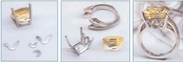
Series of photos illustrates the precision achieved with the StarWeld laser welder.
