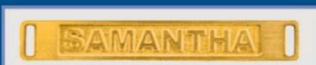
ID bracelet was engraved with the StarCut Performance at 40 mm per second. Total processing time was about 2 minutes.
