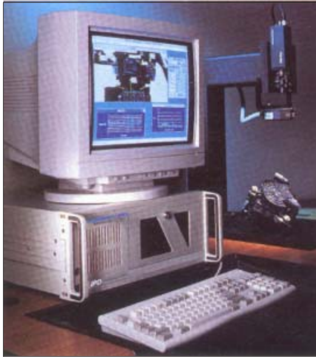
FIGURE 2. Prophecy vision system includes Pentium-based host computer, CPI bus frame grabber, and a 768 x 575 CCIR camera.
