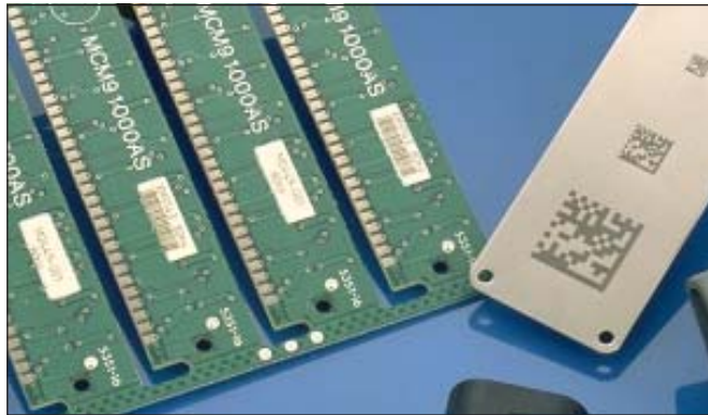
A CO 2 laser was used to remove ink from this PC Board to form a bar code. Also shown is an example of 3 different sizes of a two-dimensional matrix code.
