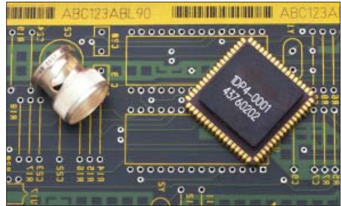
An example of text and bar codes marked on PC board by removing yellow Hysol ink using a Nd:YAG laser
